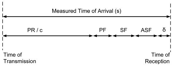
Figure 1. Components and factors affecting measured time of arrival using alternative definition of PF.
