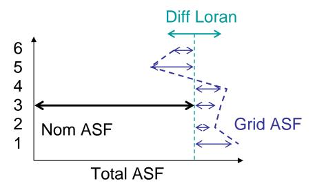
Figure 5. Definition of components to ASF
