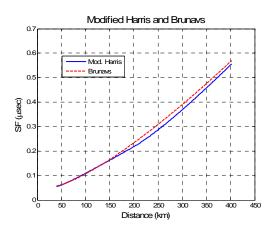
Figure 3. Two Options for Continuous SF: Modified Harris Polynomial and Brunavs (SF term only)
