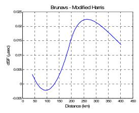
Figure 4. Difference between Secondary Factor calculated using Modified Harris Polynomial and Brunavs
